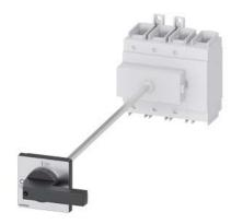
SENTRON, Switch disconnector 3LD, main switch, 4-pole, lu=250 A, Operating power / at AC-23 A at 400 V: 132 kW, floor mounting with door coupling, knob-operated mechanism, black, 4-hole mounting of the handle
