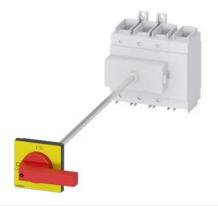
SENTRON, Switch disconnector 3LD, emergency switching-off switch, 4-pole, lu=250 A, operating power / at AC-23 A 400 V: 132 kW, floor mounting with door coupling, knob-operated mechanism, red/yellow, 4-hole mounting of the handle
