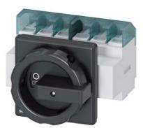
SENTRON, Switch disconnector 3LD, main switch, 6-pole, Iu: 63 A, Operating power / at AC-23 A at 400 V: 22 kW, front-mounted, rotary operating mechanism, black, 4-hole mounting of the handle
