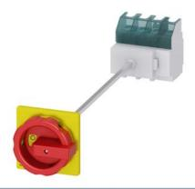
SENTRON, Switch disconnector 3LD, emergency switching-off switch, 4-pole, Iu: 63 A, operating power / at AC-23 A 400 V: 22 kW, floor mounting with door coupling, rotary operating mechanism, Red / yellow, 4-hole mounting of the handle
