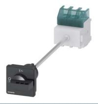
SENTRON, switch disconnector 3LD, main switch, 3-pole, lu: 63 A, operating power / at AC-23 A at 400 V: 22 kW, floor mounting with door coupling, defeatable knob-operated mechanism, black, 4-hole mounting of the handle
