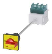
SENTRON, switch disconnector 3LD, EMERGENCY OFF switch, 3-pole, lu: 63 A, Operating power / at AC-23 A at 400 V: 22 kW, floor mounting with door coupling, defeatable knob-operated mechanism, red/yellow, 4-hole mounting of the handle
