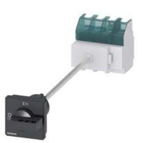
SENTRON, switch disconnector 3LD, main switch, 4-pole, lu: 63 A, operating power / at AC-23 A at 400 V: 22 kW, floor mounting with door coupling, defeatable knob-operated mechanism, black, 4-hole mounting of the handle
