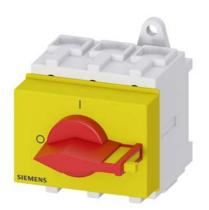
SENTRON, Switch disconnector 3LD, emergency switching-off switch, 3-pole, lu: 63 A, operating power / at AC-23 A 400 V: 22 kW, installation in distribution boards, knob-operated mechanism, Red / yellow, handle direct at the switch
