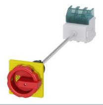
SENTRON, Switch disconnector 3LD, emergency switching-off switch, 3-pole, lu: 63 A, operating power / at AC-23 A 400 V: 22 kW, floor mounting with door coupling, rotary operating mechanism, Red / yellow, central mounting 22.5 mm of the handle
