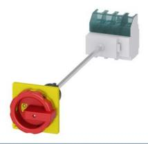
SENTRON, Switch disconnector 3LD, emergency switching-off switch, 4-pole, lu: 63 A, operating power / at AC-23 A 400 V: 22 kW, floor mounting with door coupling, rotary operating mechanism, Red / yellow, central mounting 22.5 mm of the handle
