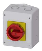
SENTRON, Switch disconnector 3LD, emergency switching-off switch, 3-pole, lu: 63 A, operating power / at AC-23 A 400 V: 22 kW, Molded plastic encapsulation for inch cable gland, 1 NC, 1 NO, rotary operating mechanism, red/yellow
