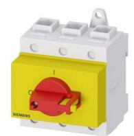
SENTRON, Switch disconnector 3LD, emergency switching-off switch, 3-pole, lu: 100 A, operating power / at AC-23 A 400 V: 37 kW, installation in distribution boards, knob-operated mechanism, Red / yellow, handle direct at the switch
