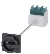
SENTRON, Switch disconnector 3LD, main switch, 3-pole, lu: 125 A, Operating power / at AC-23 A at 400 V: 45 kW, floor mounting with door coupling, rotary operating mechanism, black, 4-hole mounting of the handle
