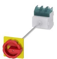
SENTRON, Switch disconnector 3LD, emergency switching-off switch, 3pole, lu: 125 A, operating power / at AC-23 A 400 V: 45 kW, floor mounting with door coupling, rotary operating mechanism, Red / yellow, 4-hole mounting of the handle
