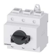
SENTRON, Switch disconnector 3LD, main switch, 3-pole, lu: 125 A, Operating power / at AC-23 A at 400 V: 45 kW, installation in distribution boards, knob-operated mechanism, black, handle direct at the switch
