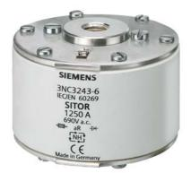
SITOR fuse link, with female thread on both sides, NH2, In: 1000 A, aR, Un AC: 690 V, Un DC: 440 V, without Indicator
