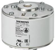
SITOR fuse link, with female thread on both sides, NH3, In: 800 A, aR, Un AC: 1100 V, Un DC: 440 V, front indicator
