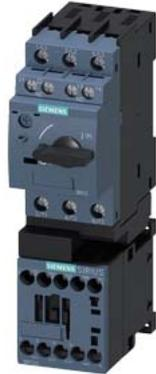
Fuseless motor starter Direct start 600VAC Size S00 7-10A 220/240VAC 50/60HZ screw connection For screw mounting Or 35 mm rail-mounting Type of coordination 1 1NO+1NC (MSP) 1NO (contactor)
