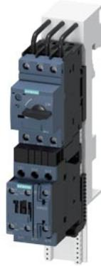
Fuseless motor starter Direct start 600VAC Size S0 4.5-6.3A 220/240VAC 50/60Hz screw connection For snapping onto 60 mm busbar systems Type of coordination 2 IQ = 150 KA Also full fills type Of coordination 1 1NO+1NC (contactor)
