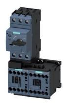
FUSELESS LOAD FEEDER REVERSING OPERATION, 400 V AC, S00 0.18 TO 0.25 A 3 KW, 110/120 V AC 50/60 HZ SCREW TERMINAL FOR STANDARD RAIL MOUNTING, TYPE OF COORDINATION 2, IQ = 150 KA (ALSO FULFILLS TYPE OF COORDINATION 1) 1NC (CONTACTOR)
