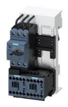
FUSELESS LOAD FEEDER REVERSING OPERATION, 400 V AC, S00 0.18 TO 0.25A 3K W, 110/120 V AC 50/60 HZ SCREW TERMINAL FOR 60 MM BUSBAR SYSTEMS TYPE OF COORDINATION 2, IQ = 150 KA (ALSO FULFILLS TYPE OF COORDINATION 1) 1NC (CONTACTOR)
