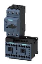
FUSELESS MOTOR STARTER REVERSING OPERATION 600V AC SZ S00 0.28-0.4A 220/240V AC 50/60HZ SCREW CONNECTION FOR SCREW MOUNTING OR 35 MM RAIL-MOUNTING TYPE OF COORDINATION 2 IQ = 150 KA ALSO FULFILLS TYPE OF COORDINATION 1 1NC (PER CONTACTOR)
