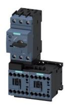
Load feeder fuseless, Reversing duty 400 V AC, Size S00 2.20...3.20 A 230 V AC screw terminal for installation on standard mounting rail (also fulfills type of coordination 1) Type of coordination 2, Iq = 150 kA 1 NC (contactor)
