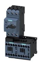
Load feeder fuseless, Reversing duty 400 V AC, Size S00 4.50...6.30 A 230 V AC screw terminal for installation on standard mounting rail Type of coordination 1, lq = 150 kA 1 NC (contactor)
