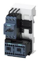
Load feeder fuseless, Reversing duty 400 V AC, Size S00 7.00...10.0 A 230 V AC screw terminal for 60 mm busbar systems Type of coordination 1, Iq = 150 kA 1 NC (contactor)
