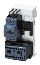
Load feeder fuseless, Reversing duty 400 V AC, Size S00 9.00...12.5 A 230 V AC screw terminal for 60 mm busbar systems Type of coordination 1, Iq = 150 kA 1 NC (contactor)
