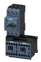
FUSELESS LOAD FEEDER REVERSING OPERATION, AC 400V, S00 10...16A, AC 110/120V 50/60HZ SCREW TERMINAL FOR RAIL MOUNTING, TYPE OF ASSIGNMENT 1,IQ = 150KA 1NC (CONTACTOR)
