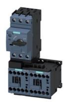
Load feeder fuseless, Reversing duty 400 V AC, Size S00 10.0...16.0 A 230 V AC screw terminal for installation on standard mounting rail Type of coordination 1, Iq = 150 kA 1 NC (contactor)
