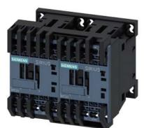
reversing contactor assembly, AC-3e/AC-3, 9 A, 4 kW / 400 V, 3-pole, 230 V AC, 50/60 Hz, spring-loaded terminal, electrical and mechanical interlock
