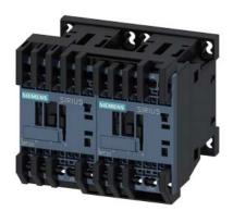
reversing contactor assembly, AC-3e/AC-3, 16 A, 7.5 kW / 400 V, 3-pole, 230 V AC, 50/60 Hz, spring-loaded terminal, electrical and mechanical interlock
