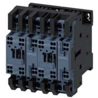
reversing contactor assembly, AC-3e/AC-3, 12 A, 5.5 kW / 400 V, 3-pole, 110 V AC, 50/60 Hz, spring-loaded terminal, electrical and mechanical interlock, auxiliary contacts:  $2 \times 1 \text{ NO}$
