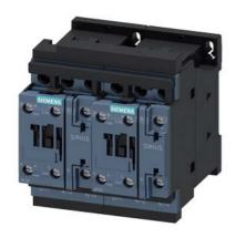
reversing contactor assembly, AC-3e/AC-3, 17 A, 7.5 kW / 400 V, 3-pole, 220 V AC, 50 Hz / 240 V, 60 Hz, screw terminal, electrical and mechanical interlock, auxiliary contacts: 2 x 1 NO
