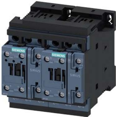
reversing contactor assembly, AC-3e/AC-3, 17 A, 7.5 kW / 400 V, 3-pole, 24 V DC, screw terminal, electrical and mechanical interlock, auxiliary contacts: 2 x 1 NO, with voltage tap for 3RA27
