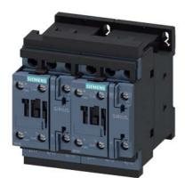
reversing contactor assembly, AC-3e/AC-3, 32 A, 15 kW / 400 V, 3-pole, 110 V AC, 50/60 Hz, screw terminal, electrical and mechanical interlock, auxiliary contacts: 2 x 1 NO
