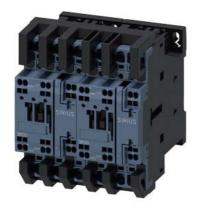
reversing contactor assembly, AC-3e/AC-3, 32 A, 15 kW / 400 V, 3-pole, 230 V AC, 50/60 Hz, spring-loaded terminal, electrical and mechanical interlock, auxiliary contacts: 2 x 1 NO
