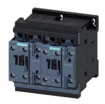
reversing contactor assembly, AC-3e/AC-3, 38 A, 18.5 kW / 400 V, 3-pole, 24 V AC, 50/60 Hz, screw terminal, electrical and mechanical interlock, auxiliary contacts:  $2\times1$  NO
