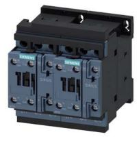
reversing contactor assembly, AC-3e/AC-3, 38 A, 18.5 kW / 400 V, 3-pole, 230 V AC, 50/60 Hz, screw terminal, electrical and mechanical interlock, auxiliary contacts: 2 x 1 NO
