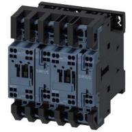
reversing contactor assembly, AC-3e/AC-3, 38 A, 18.5 kW / 400 V, 3-pole, 230 V AC, 50/60 Hz, spring-loaded terminal, electrical and mechanical interlock, auxiliary contacts: 2 x 1 NO
