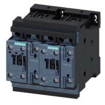
reversing contactor assembly, AC-3e/AC-3, 38 A, 18.5 kW / 400 V, 3-pole, 24 V DC, screw terminal, electrical and mechanical interlock, auxiliary contacts: 2 x 1 NO, with voltage tap for 3RA27
