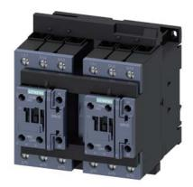
reversing contactor assembly, AC-3e/AC-3, 41 A, 18.5 kW / 400 V, 3-pole, 230 V AC, 50/60 Hz, screw terminal, electrical and mechanical interlock, auxiliary contacts: 2 x 1 NO
