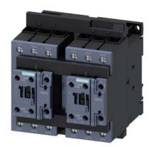
reversing contactor assembly, AC-3e/AC-3, 51 A, 22 kW / 400 V, 3-pole, 110 V AC, 50/60 Hz, screw terminal, electrical and mechanical interlock, auxiliary contacts: 2 x 1 NO
