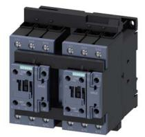
reversing contactor assembly, AC-3e/AC-3, 51 A, 22 kW / 400 V, 3-pole, 20-33 V AC/DC, 50/60 Hz, screw terminal, electrical and mechanical interlock, auxiliary contacts: 2 x 1 NO
