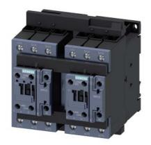
reversing contactor assembly, AC-3e/AC-3, 51 A, 22 kW / 400 V, 3-pole, 20-33 V AC/DC, 50/60 Hz, screw terminal, electrical and mechanical interlock, auxiliary contacts: 2 x 1 NO, with voltage tap for 3RA27
