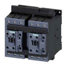
reversing contactor assembly, AC-3e/AC-3, 65 A, 30 kW / 400 V, 3-pole, 20-33 V AC/DC, 50/60 Hz, screw terminal, electrical and mechanical interlock, auxiliary contacts: 2 x 1 NO, with voltage tap for 3RA27
