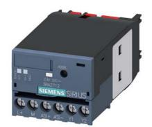
Function module for AS-i, direct start, screw terminal, Installation on contactors 3RT2 Communication-capable contactor required
