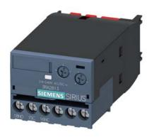
Solid-state time-delayed auxiliary switch ON delay Relay 1 changeover contact 24...240 V AC/DC Time range 0.05...100 s Can be snapped on at the front For 3RT2 S00-S3 contactors and 3RH2 S00 contactor relays Screw terminal Varistor for attenuation of the contactor coils integrated
