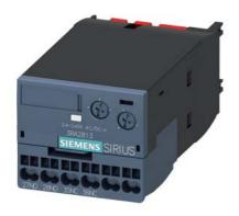
solid-state time-delayed auxiliary switch, ON-delay, relay 1 NC + 1 NO, time range 0.05-100 s, 24-240 V AC/DC, 50/60 Hz, varistor for attenuation of the contactor coils integrated, spring-loaded terminal, can be snapped on at the front on contactors 3RT2 and auxiliary contactors 3RH2
