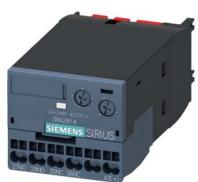
solid-state time-delayed auxiliary switch, off delayed, with control signal, relay 1 NC + 1 NO, time range 0.05-100 s, 24-240 V AC/DC, 50/60 Hz, varistor for attenuation of the contactor coils integrated, spring-loaded terminal, can be snapped on at the front on contactors 3RT2 and auxiliary contactors 3RH2
