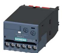
solid-state time-delayed auxiliary switch, off delayed, without control signal, relay: 1 CO, time range 0.05-100 s, 24-240 V AC/DC, 50/60 Hz, varistor for attenuation of the contactor coils integrated, screw terminal, can be snapped on at the front on contactors 3RT2 and auxiliary contactors 3RH2
