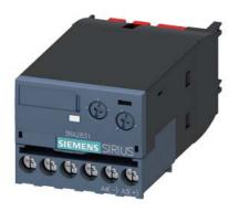
electronic timing relay, ON-delay, with semiconductor output, time range 0.05-100 s, 24-90 V AC/DC, 50/60 Hz, varistor for attenuation of the contactor coils integrated, screw terminal, can be snapped on at the front on contactors  $3RT2.3\,/\,3RT2.4$
